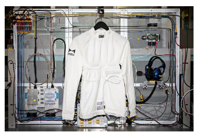
VISM allows real time monitoring of the driver's state of health through the elaboration of ECG (electrocardiogram) and thoracic expansion, both acquired by the sensors. The simultaneous analysis of heart rhythm and breath rate allows the driver performance index to be monitored in real-time, and so immediately identify possible states of stress, fatigue and alteration.
